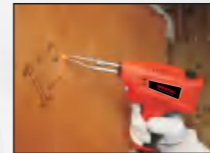
Area C: 350°C-500°C Engraving on wood
